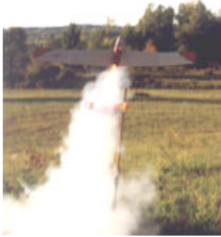
Third and final flight. 1/10 second before catastrophic failure. A crack in the motor is already directing the flame toward the v-tail
