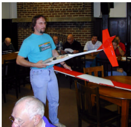
Tom Koszuta with Thermal Plane Modified for Slope with MH42 Airfoil
